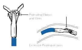
Accessories with protruding components can cause excessive biopsy channel damage and result in substantial scope repair costs.
