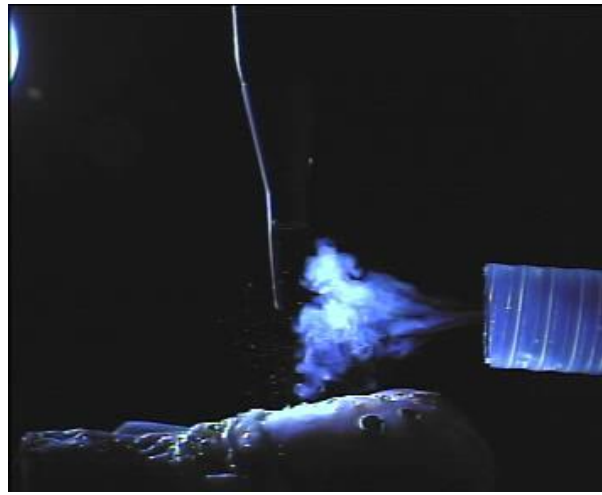
Figure 7. The pulsed CO 2 laser creates explosive smoke plumes and aerosol. The smoke is effectively removed. However, the aerosols are ejected at high speed from the source
